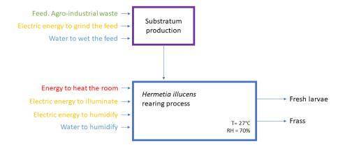
Figure 2. Process system to generate frass and BSF.
