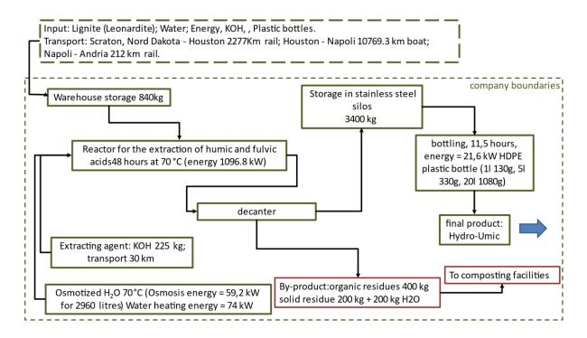
Figure 1. Production cycle of Lignite-based biostimulants BL.
